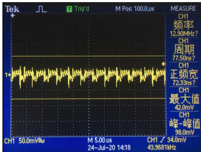
Noise (VIN = 48V, IO = 2A, 5 ~ 20MHz bandwidth)
